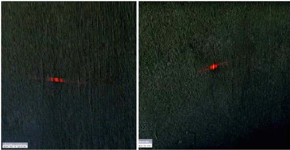
Fig. 7 At the left and right subfigures we see photographs of the optical single-slit diffraction pattern taken at the start of the experiment from the spurious double-slit screen where the true nature of this screen was known and used during the experiment. The distance between the mirror and wall, used for obtaining the optical pattern of the left picture , was larger compared to that used for the right picture
