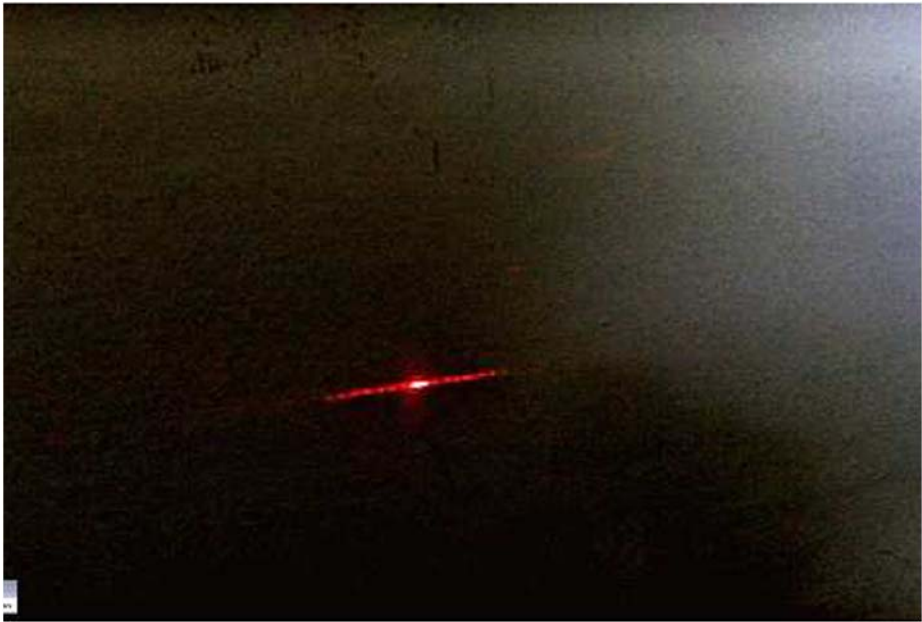
Fig. 8 This figure is a photograph of the optical interference pattern obtained from the spurious double-slit screen where the true nature of this screen was not known and, therefore, not used during the experiment. Note the similarity of this pattern, actually obtained from single-slit screen, to that of Fig. 6 which was obtained from one of the real double-slit screens. Comparing this photograph to those of Fig. 7, which are obtained from the same screen, one may realize that the use (or not) during the experiment of the relevant data is the important factor which determines the obtained optical pattern
